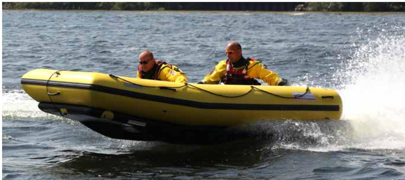
The RC4000 Rescue Craft is designed to exceed the performance of a conventional Inflatable flood rescue boat, while providing the shallow draft and ease of transportation of a rescue sled. The inflatable four meter design with twin keels and a rigid inflatable floor represents the latest thinking in flood rescue boat design.
