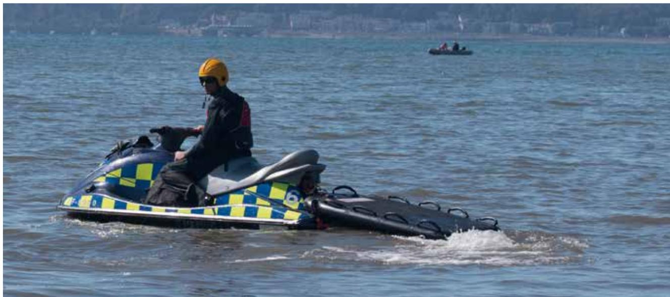
The Jet Ski Rescue Board is an inflatable board that is designed to be attached to the back of a jet ski to aid rapid response and rescue of casualties. It is attached by a towing 'D' ring and two other 'D' rings which are located at the front of the inflatable board.
