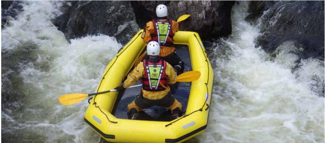
Fully inflatable, the Evacuation Raft is lightweight and portable. It is easy to manoeuvre, and can be paddled or pulled by hand. The Evacuation Raft has a flat bottom, making it exceptionally stable and suitable for use in very shallow water from 50mm in depth. The Evacuation Raft is ideal in flood rescue situations.
