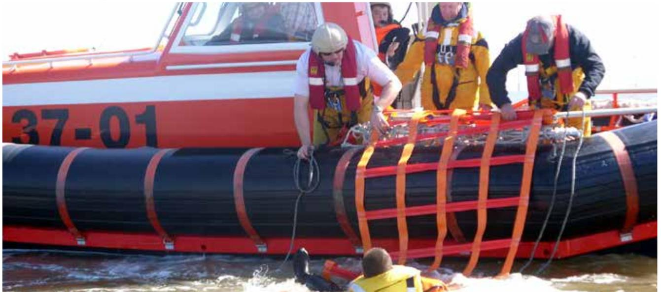
The Fibreight Cradle is a SOLAS approved 'Man Overboard Recovery Device' that has the versatility to recover casualties into many different types and sizes of vessels.
