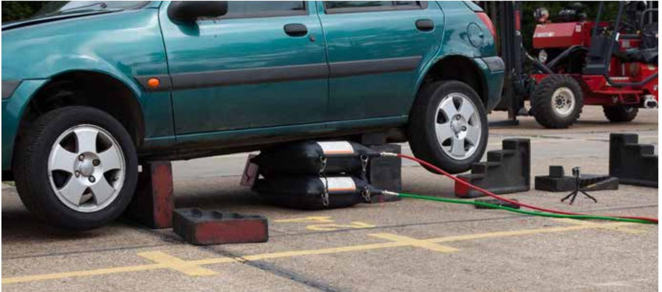
The Stak Jak is a revolutionary flat-profile lifting cushion for vehicle and heavy duty lifting requirements. The flat profile of the Stak Jak has several distinct advantages over traditional ovoid lifting cushions of which the most significant is the ability to safely stack up to three cushions together. This enables a greater lift height without the risk of sudden ejection or instability that is possible when stacking ovoid mats.
